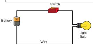
**Electricity** can only flow around a complete circuit that has no gaps. There must be wires connected to both the positive and negative end of the power supply/battery.
